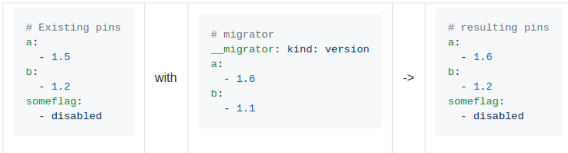
Figure 5. Simple version migrator used to update configuration YAML files. Original file on the left, migrator in the middle, and resulting file on the right. Tags are only updated if the version number is greater than the original version number.
